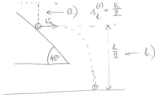
a) in case of the first half of the movement  $\rightarrow$  free fall:  $\rightarrow$   $v_0=0$
