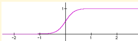
Figure 6: Unipolar activation function.
