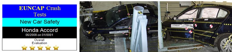
Figure 12 Honda accord 2008 EUNCAP side pole crash test [12]
