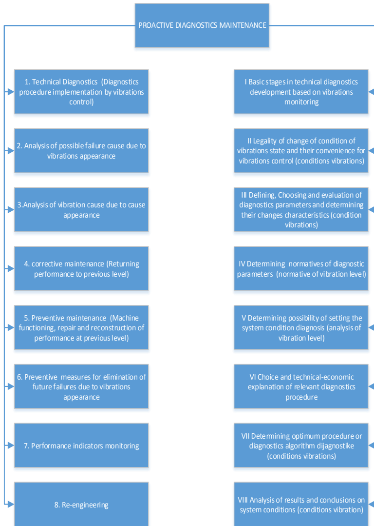
Figure 3 Model of proactive diagnostic maintenance
