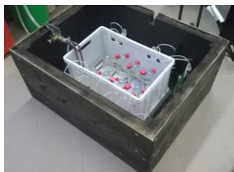
Figure 3. Custom designed water tempered bioreactor block with internal stirring
